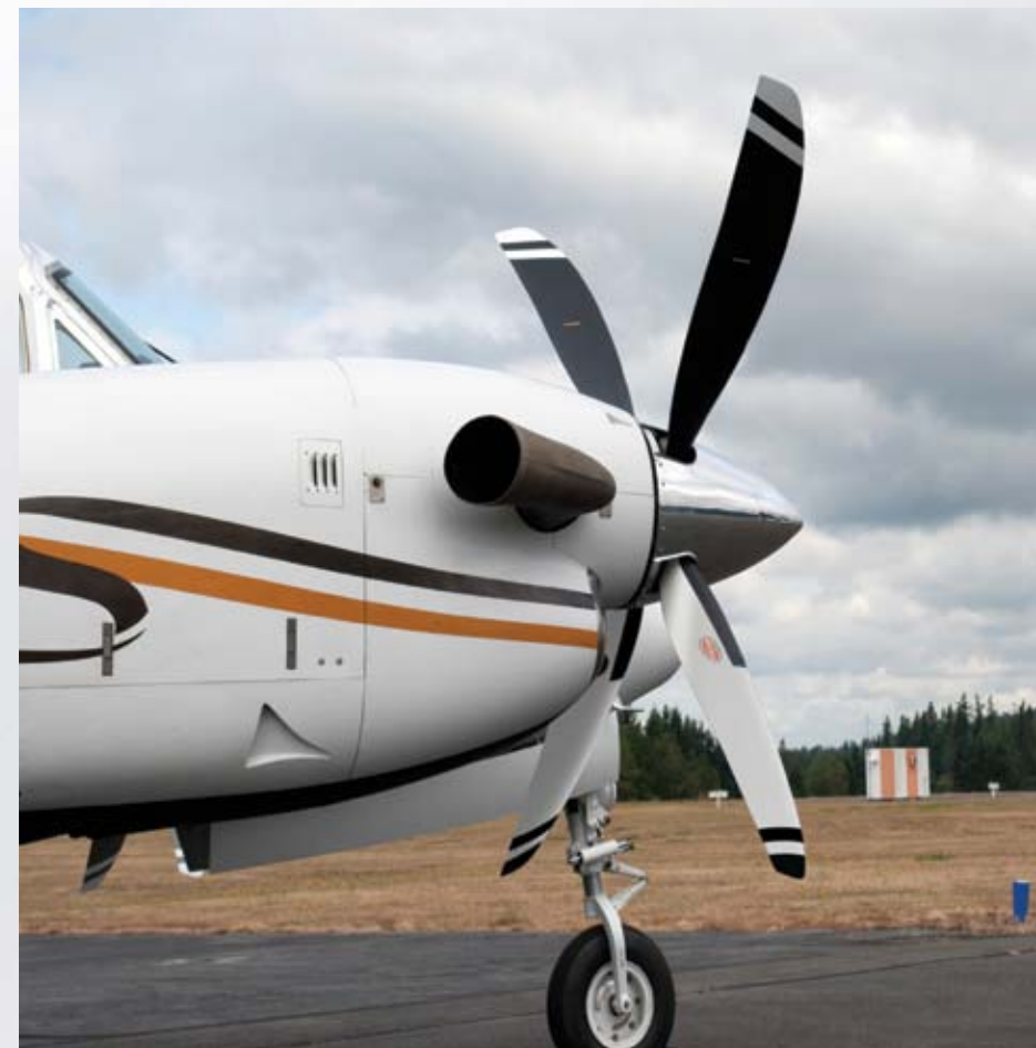
Raisbeck Swept Blade Turbofan Propellers installed on a King Air B200
