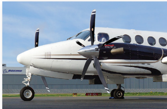
Composite 5-Blade Swept Propellers for 300, B300, 350 Benefits: Unlimited blade life; more thrust; less noise; 6-yrs/4,000 hrs TBO
