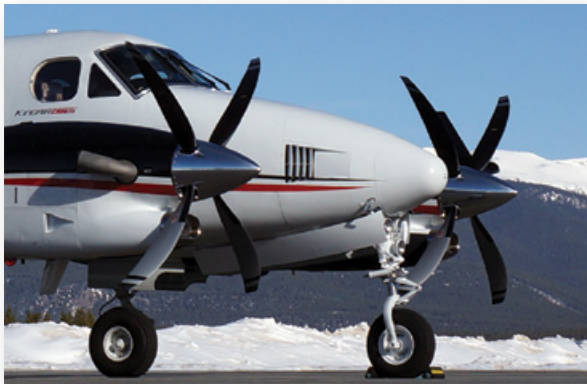
Aluminum 4-Blade Swept Propellers for C90 (All), E90 Benefits: More thrust; less noise and vibration; 6-yrs/4,000 hrs TBO Autofeather required
