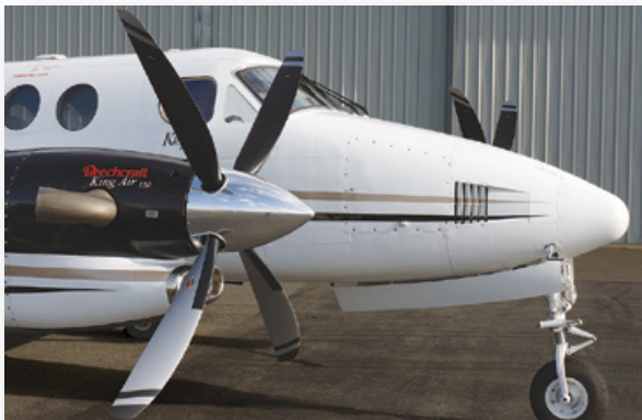
Aluminum 4-Blade Swept Propellers for 300, B300, 350 Benefits: More thrust; less noise and vibration; 6-yrs/4,000 hrs TBO
