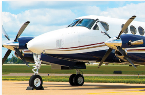
Aluminum 4-Blade Swept Propellers for 200, B200, B200GT, 250 Benefits: More thrust; less noise and vibration; 6-yrs/4,000 hrs TBO Autofeather required
